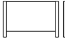
5054 Double Bed w/ Bolt On Spring 55" wd x 78" lg x 36" hi - Accepts 54" x 76" mattress
